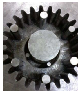
Figure.6 The die holes for ejectors
