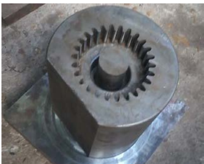
Figure.5 The die after milling
