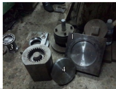
Figure.7 The die parts 1-base of die 2-bearing holder 3-rod 4-Cover of Die
